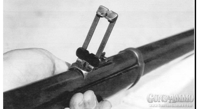
The rear ladder sight was graduated to 1,400 yards, though authorities found long-range accuracy with the Martini-Henry to be disappointing.
