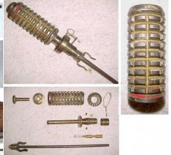
Above; Hales rifle grenade complete and disassembled components.
