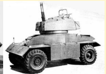
Below; AA Turreted ACE car with twin 20mm Oerlikon
