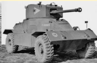
Below; Mk III Close Support Car with QF 75 mm gun
