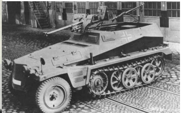
Above; is Sd.kfz250/11 half-track mounting a 2.8 cm schwere Panzerbüchse 41
