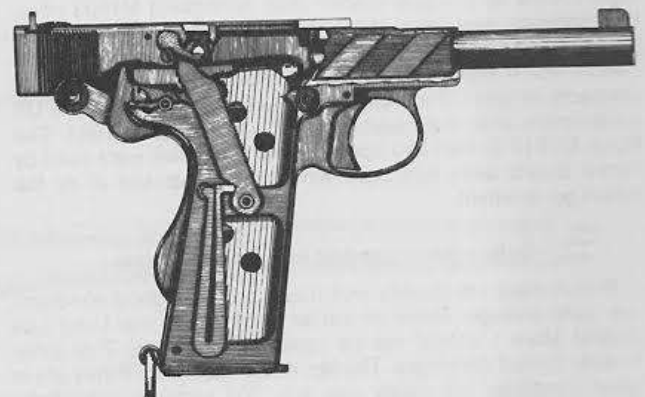
Action open and cutaway to show mainspring and sear.
