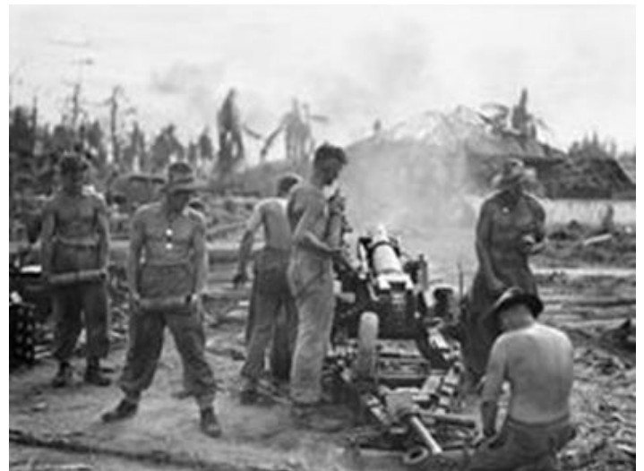
A 2/4th Short 25-pounder firing at Balikpapan, July 1945 Left is a Australian Baby/Short 25-pounder, which was designed in 1942 and entered service 1943 for jungle warfare. Used by Australian Army and some US Army units.
