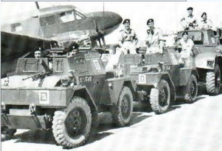
Two Daimler Mk I Scout Cars and a Mk II Armoured Car at the back
