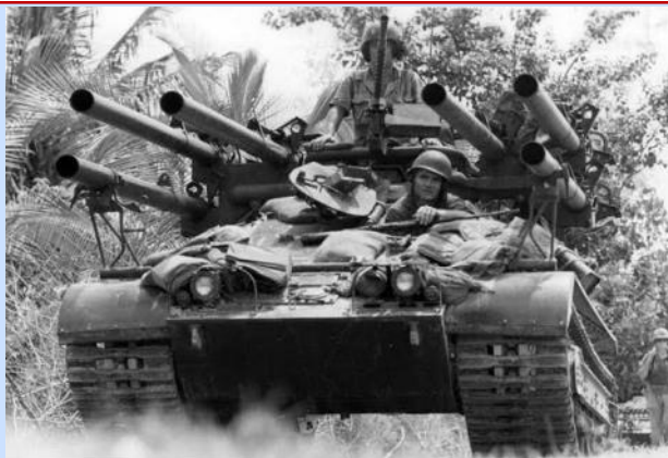
Ontos M50A1, the 50-cal spotting rifles can be seen on the upper guns
