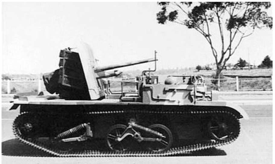
2 pounder guns mounted on modified Australian-built Carrier
