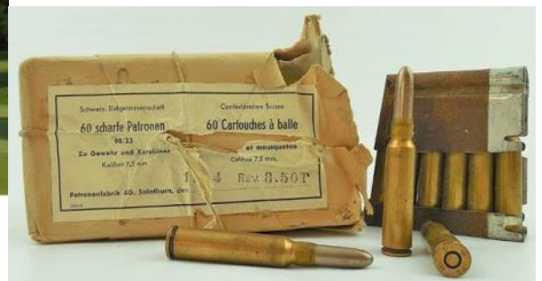
Left and Above Left is Alecto MK 3 Below Packet of military 7.5x53.5mm GP 90/23 Ammo With a cardboard Stripper Clip
